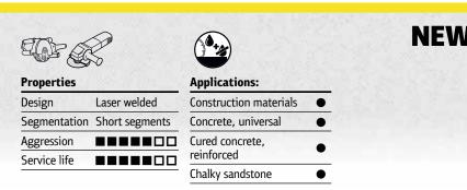
**Advantages:** Suitable for a various range of applications - First-rate cutting performance - Exceptional service life thanks to the use of premium grade raw materials and diamonds - Clean cutting edges
