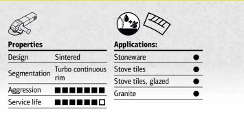
**Advantages:** 1/16 " thin professional blade for extremely demanding applications - Work results of superior quality - Continuous rim with turbo segments - Clean and nick-free edges
