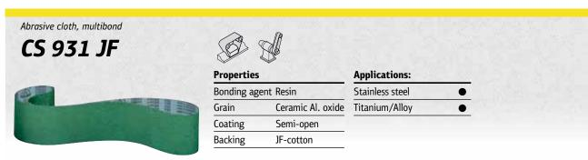
**Advantages:** Special product with high flexible backing for the processing of stainless steel and high-alloyed steel - Continuously aggressive grinding properties with high lifetime due to semiopen coated self-sharpening ceramic grain - Very good adaptability to radiuses and edges through high flexible backing - The additional multibond provides a "cool grinding" in the processing of stainless steel and thus tempering colours are avoided
