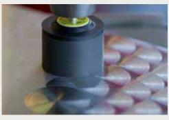
Example of a decorative finish created with an R-Flex mottling point SFM 656 on a stainless steel sheet
