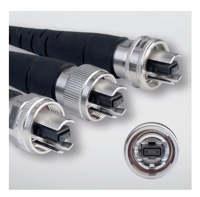
Precisely polished MT ferrules ensure the excellent contact of all twelve parallel optical fibers, which is verified by regular interferometer testing. The ferrules are available in the standard physical contact version for multimode fibers and in an 8° angled physical contact version for even better return loss performance with singlemode fibers.
