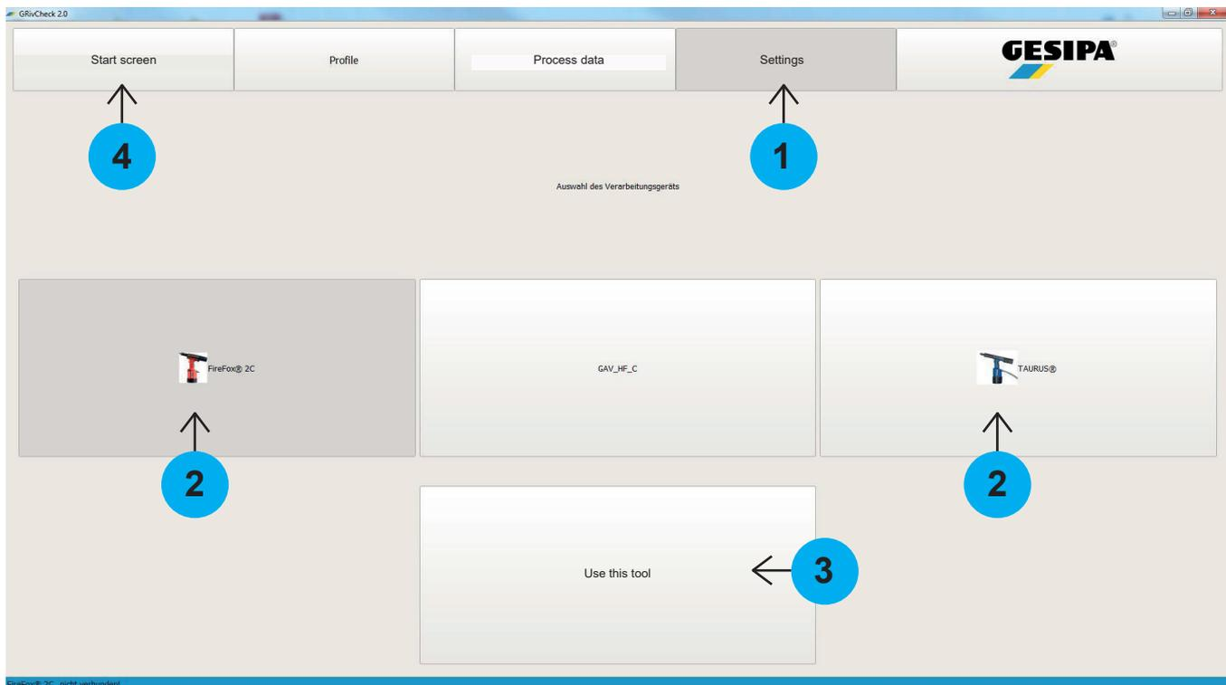
Now the tool has to be connected (1). The connection status is displayed in the task bar (2)
