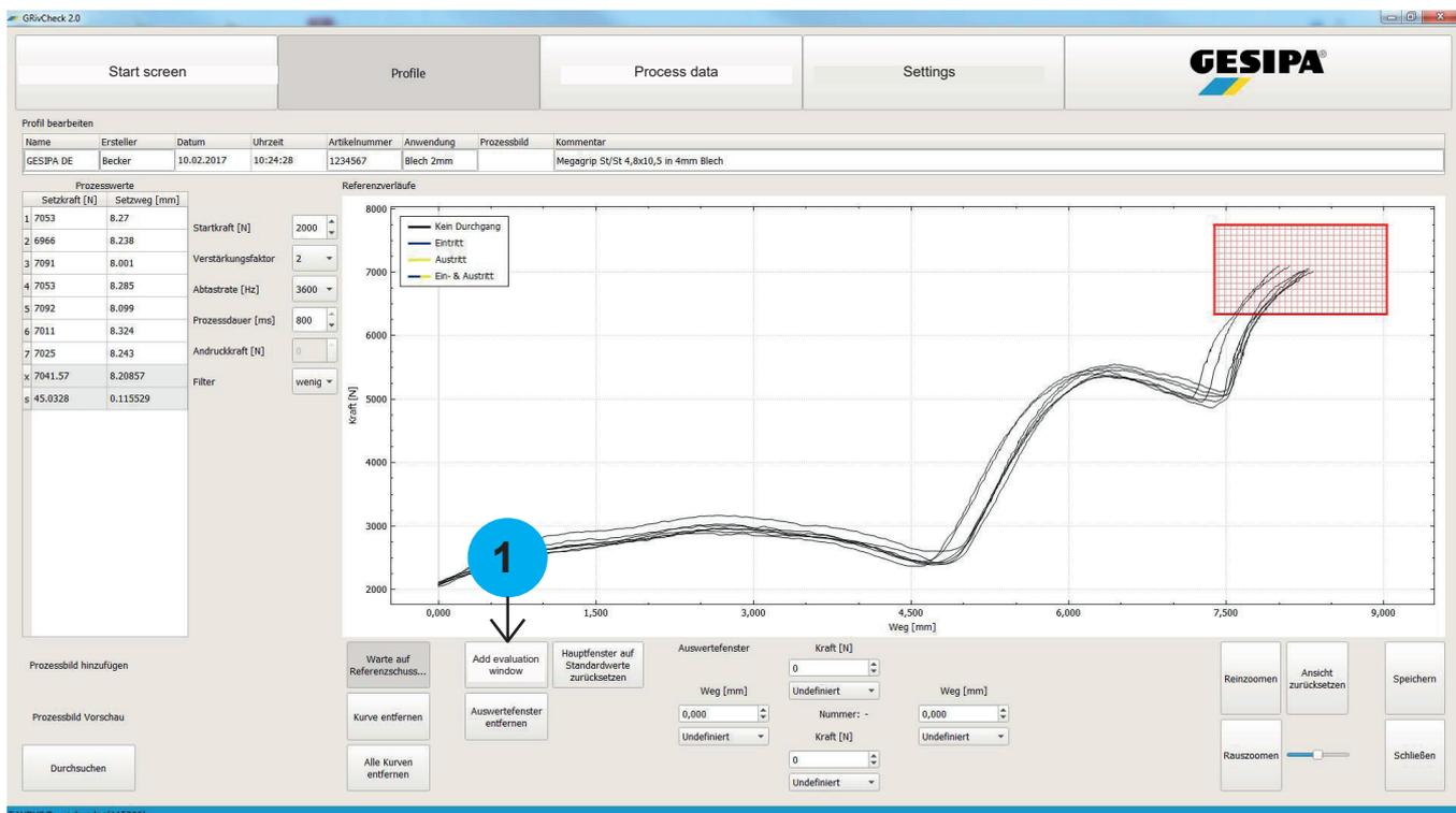
The evaluation window has to be defined. To do this, select the evaluation window and choose its size. The window pages have to be defined in the lower menu (1). Once the window is defined, an NOK riveting procedure can be performed (e.g. component forgotten, rivet incorrectly inserted into component, component inserted too much, etc.)
