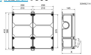
Standard cable entries pre-punched Top: 1xM12, 1xM20, 2xM40 Bottom: 1xM12, 1xM20, 2xM40
