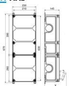
Standard cable entries pre-punched Top: 1xM12, 1xM20, 2xM40 Bottom: 1xM12, 1xM20, 2xM40
