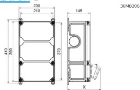
Standard cable entries pre-punched Top: 1xM12, 1xM20, 2xM40 Bottom: 1xM12, 1xM20, 2xM40
