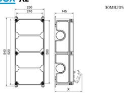
Standard cable entries pre-punched Top: 1xM12, 1xM20, 2xM40 Bottom: 1xM12, 1xM20, 2xM40
