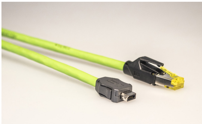
Fig. 3: Two data connectors in two sizes: RJ45 with 8 pins and ix Industrial™ with 8 plus 2 pins
