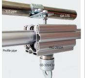
The B-044B is used to connect two profile pipes. It thus makes it possible to use it as a guide rail for trolleys. Attached to the SUS pipe is the GA-15S joint set which connects the basic joint B-044B by a screw M6. The profile pipe is held in the middle by the B-044B, on which the flexible pipe guide rail PRG-2810A is mounted.
