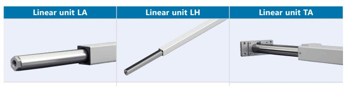
The housing of the linear unit consists of colourless anodised aluminium profile (35 x 35 mm). The tube (Ø25 mm) made of stainless steel stainless steel is mounted in a plastic mounted in a plastic bush.
