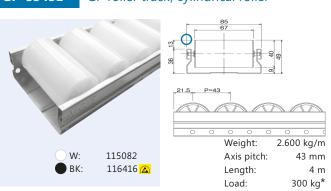
GP roller track, coated cylindrical roller GP-8550SR1
