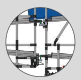
The MC-SFS is triggered by frontal drive-up to the rack. After docking the bolt is pushed down and the containers are released and move independently.
