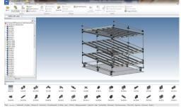
Example of a 3D drawing with the individual elements in the structure tree (left) and standard elements in the catalogue (below).
