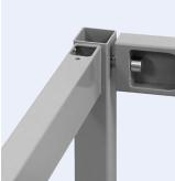
The construction principle: crossbars of the requested width are fastened to the securely welded side parts using a stable M12 bolt connection.
