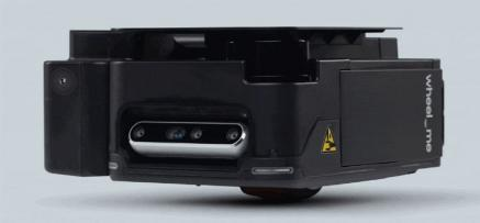
The Genius 2 module from wheel.me transforms shelves, trolleys, pallets and more into fully-fledged autonomous mobile robots (AMR).
