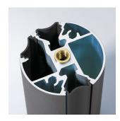
The Swing profile has just three cut-outs: two segments opposite each other are used for connection purposes and another is used for the cable duct. In the centre of the profile, levelling screws are mounted at the bottom and adapters for lights and pivoting arms are mounted at the top.
