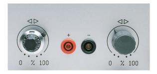
The use of multi-turn potentiometers allows for the voltage to be adjusted finely in conjunction with a digital instrument. A multi-turn potentiometer can also be installed for use in adjusting the current.
