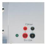
The LED status display signals short circuits and excess current as well as notifying you if surge or thermal protection is being applied. Sensor leads can be connected to compensate for the voltage drop in the leads during a 4-wire measurement process. This is important in particular in the case of test items or assemblies with a low supply voltage and high current.
