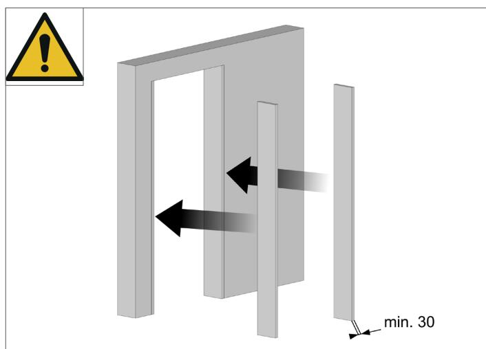
Fix out of plumb opening e. g. with 30 mm Multiplex. For calculations see page 7.
