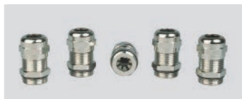
HSK MS-E-D Mosiądz IP 68, 10 bar, temp. -40°C/+100°C
