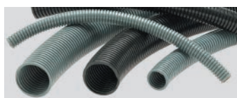
Helucond PA6 350N UL94 V2, temp. -40°C/+120°C
