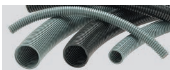
Helucond PA6-L 250N UL94 V2, temp. -40°C/+120°C
