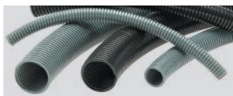
Helucond PA6 350N UL94 V2, temp. -40°C/+120°C
