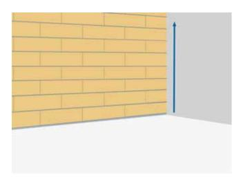
**Adjacent building elements** such as ceilings, wooden beams or windows should be prepared and masked off with airtight, pre-compressed PU soft foam sealing tape, Compriband 15/5-10, for subsequent decompression. Use the tear-off foil to control the activation time.
