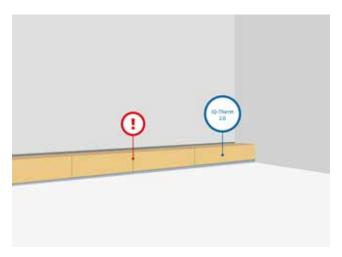
Leave joints clear between the strips. Avoid creating cross joints. Align using a straightedge.
