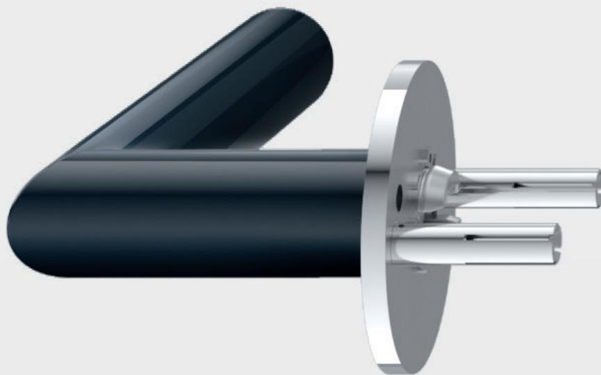
The innovative mounting technology of the flat rose enables extremely fast and permanent fixing without screws. For the fixing, latching sleeves and threaded bolts are pushed into each other, so that they lock together and are pull-resistant. The quick connection makes installation and dismantling simple. Fire door fitting sets to DIN 1827 complete the projects range.
