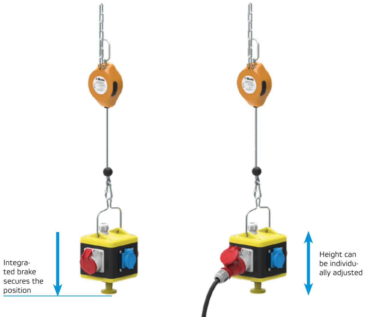
With the positioner, the risk of injury posed by hanging supply units is greatly minimised. Depending on the use, the height of the suspended unit can be conveniently varied. The integrated brake ensures that the position is securely held in place – even if the weight is changed, e.g., by plugging in or unplugging compressed air hoses. The housing, manufactured from a special plastic, is extremely impact resistant and is, thus, also suitable for use in very harsh production environments.
