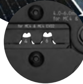
The crimping dies for 4 and 6 mm 2 crimp the standard MC4® – and the even more robust MC4® Evo 2 plug type connectors
