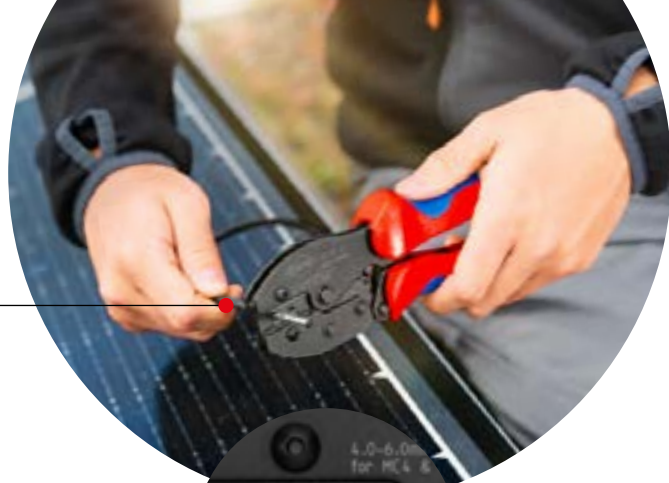
The crimping dies for 4 and 6 mm 2 crimp the standard MC4® – and the even more robust MC4® Evo 2 plug type connectors
