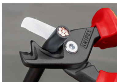
Stepped cutting edges prevent cables from slipping out
