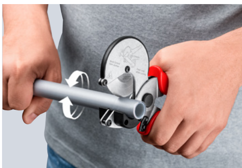
Makes cutting particularly easy: the rotating cutting wheel allows the pipe to be rotated in the pipe cutter with little friction, or, vice versa, the pipe cutter can be rotated around the pipe
