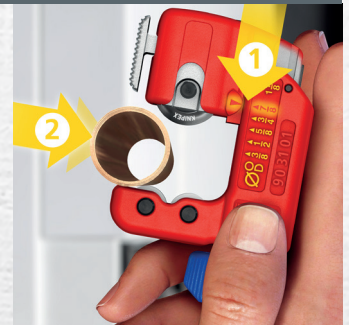
... preset with the scale and click onto the tube with the spring-loaded cutting wheel
