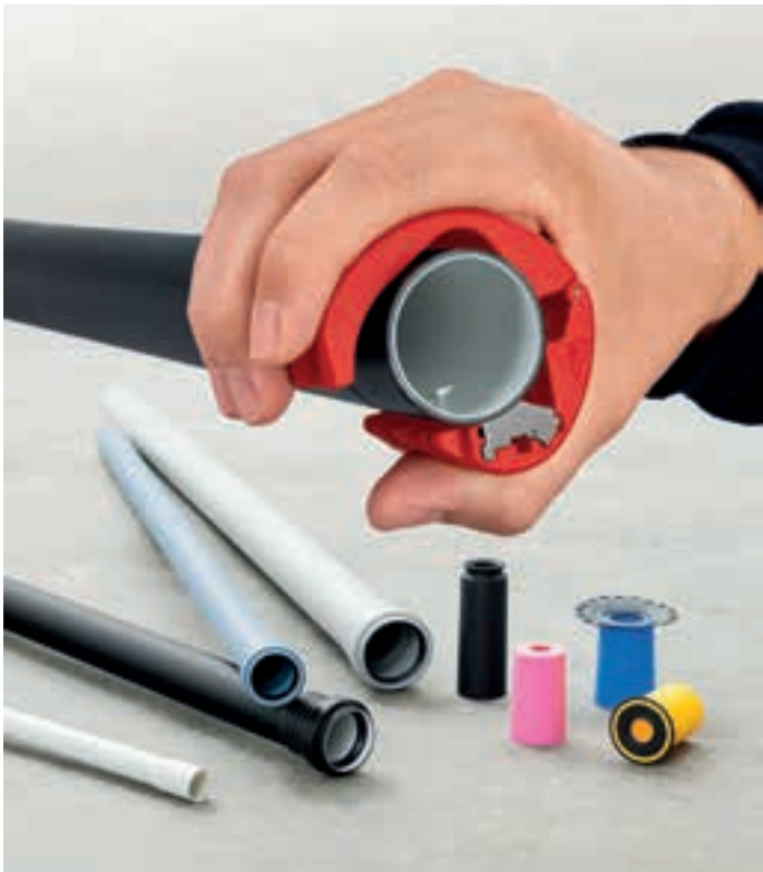
The unique design of the rotating blade unit means that drip and sealing sleeves can be reliably cut 2 to 3 mm from the wall, so that moisture can be safely drawn away
