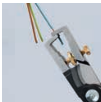
Length mark: Profiling on the inner side helps when stripping wire in standard lengths (11 mm and 16 mm)
