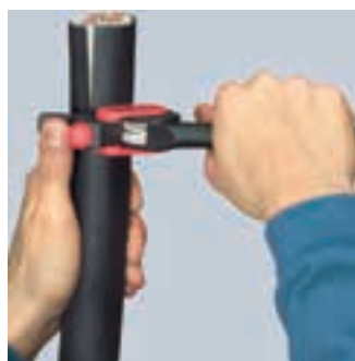
Turning the tool for circumferential cut
