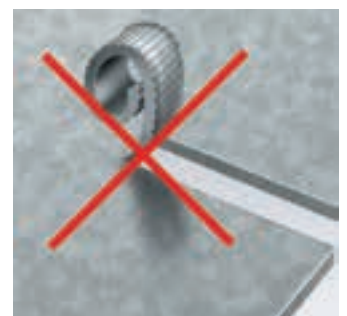
Notching without chip breaking
