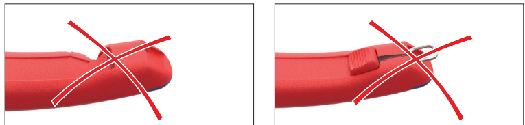
Figure 16: Do not use the TetheredTool Clip if the handle of the tool is damaged
