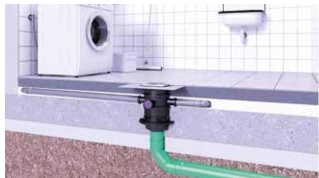
Installation with waterproofing against groundwater
