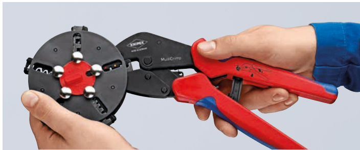
Changing the crimping dies: unlock the magazine position, take out the set of dies which the pliers have been pushed on
