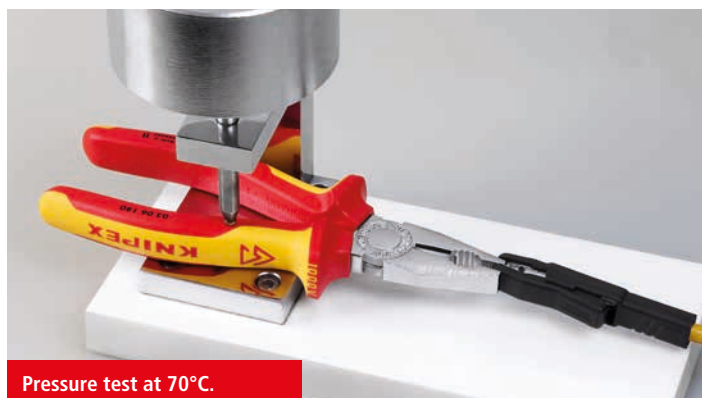
Testing the adhesion of the VDE insulating grips with 500 N at 70° C.
