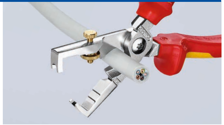
Induction hardened shear blade with precisely ground cutting edges for crushing-free cutting of copper cables of up to Ø 15 mm (5 x 2.5 mm 2 )
