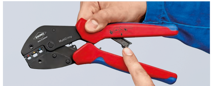
Fold in the service lever and press the pliers – ready for use again
