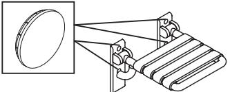
39006<br>68556 | <b>HEWI Masking cap</b><br><b>for hinged support rail 801.50... and hinged seat 801.51...</b><br>· two caps to cover the fixing points<br>· ø 23 mm<br>· delivery in pairs<br>· made of high-quality polyamide in 12 HEWI colours**<br>· made of high-quality matt polyamide in HEWI colours<br>99 (pure white), 98 (signal white), 97 (light grey), 95 (stone grey)<br>and 92 (anthracite grey)<br>Please advise colour when ordering. |
