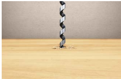
Bohren in Holz
