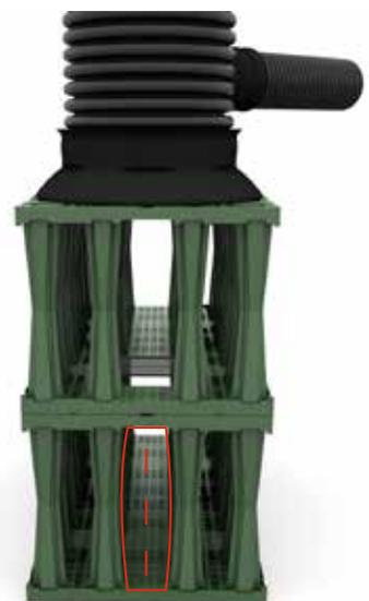
Rigofill ST can be cleaned with a flushing pressure of approx. 90 - 120 bar. The flush water transports the dirt to the control shaft QuadroControl ST and is sucked off there. It is recommended to use a 90 ° rotating nozzle with additional 45 ° rotation angle.
